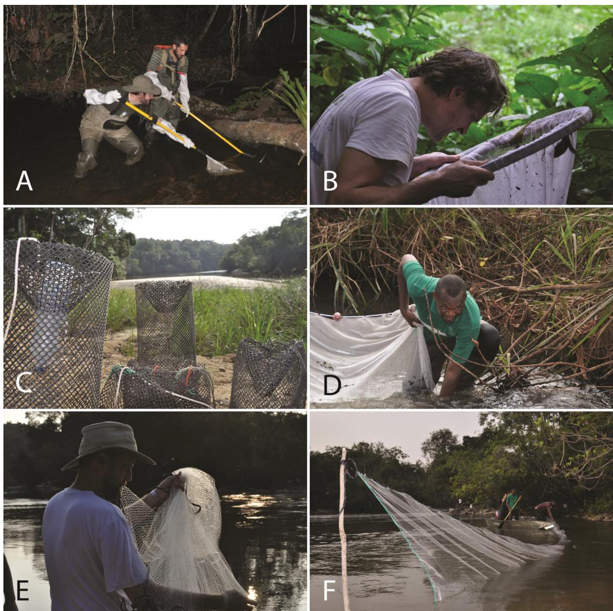
**Figure 3.** Sampling Equipment. **A.** Halltech HT-2000 backpack electroshocker and dip net. **B.** Bicycle wheel dip net. **C.** Trap. **D.** Seine net. **E.** Cast net. **F.** Gill net.
